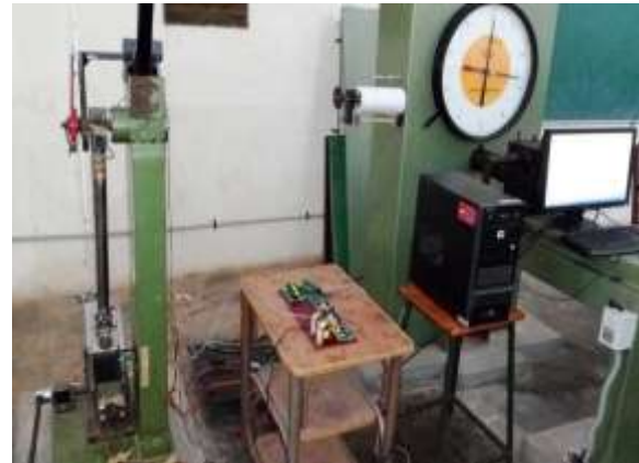
Fig. 5. Instrumented impact testing setup
